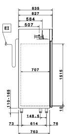
El = Electrical inlet (power) RI = Refrigerant Inlet = Refrigerant Outlet
